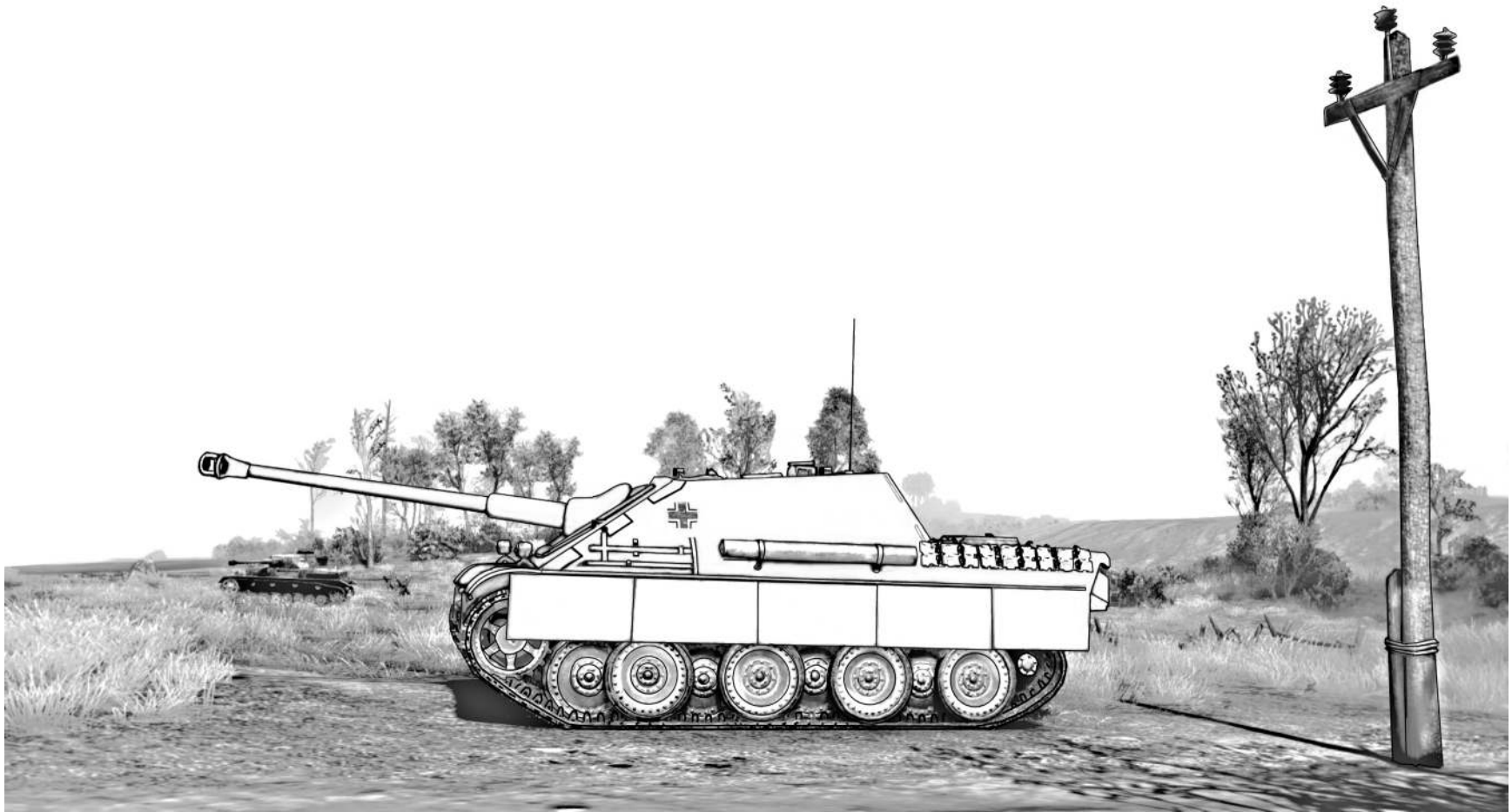
(12) Jagpanther. A tank destroyer featuring the powerful 8.8cm PaK 43 main gun mounted on a Panther chassis.
